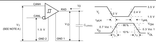
A. The input pulse is supplied by a generator having the following characteristics: PRR  $\leq$  125 kHz, 50% duty cycle,  $t_r \leq$  6 ns,  $t_f \leq$  6 ns,  $Z_O =$  50  $\Omega$ .
