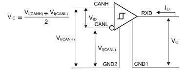
Figure 7-4. Receiver Voltage and Current Definitions
