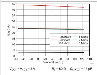
Figure 6-7. I<sub>CC2</sub> vs Ambient Temperature for Recessive, Dominant and Different CAN Datarates
