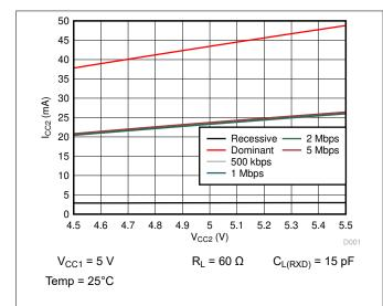
Figure 6-5. I<sub>CC2</sub> vs V<sub>CC2</sub> for Recessive, Dominant and Different CAN Datarates
