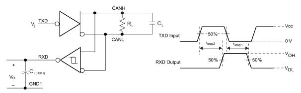
Figure 7-6. t<sub>LOOP</sub> Test Circuit and Voltage Waveforms
