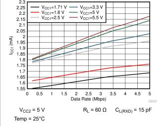
Figure 6-6. I<sub>CC1</sub> vs Datarate
