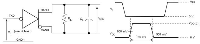
A. The input pulse is supplied by a generator having the following characteristics:  $t_r \le 6$  ns,  $t_f \le 6$  ns,  $Z_O = 50$   $\Omega$ .
