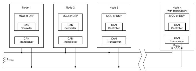
Figure 9-3. Typical CAN Bus
