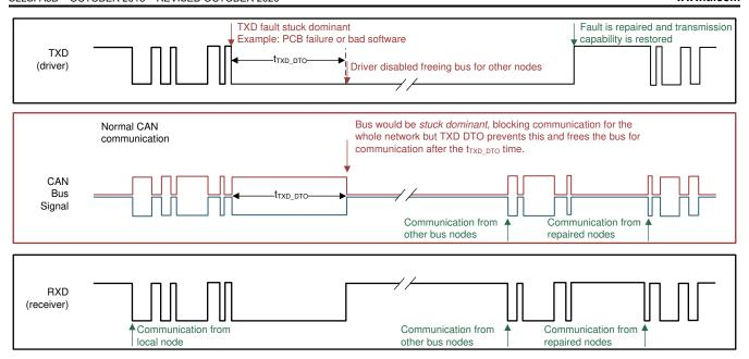
Figure 8-3. Example Timing Diagram for TXD DTO
