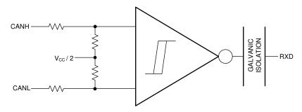
Figure 8-2. Simplified Recessive Common Mode Bias and Receiver
