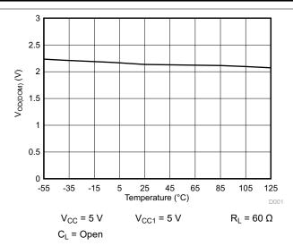
Figure 6-10. V<sub>OD(DOM)</sub> Over Temperature
