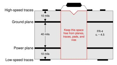
Figure 11-1. Recommended Layer Stack
