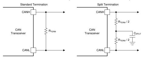
Figure 9-4. CAN Bus Termination Concepts
