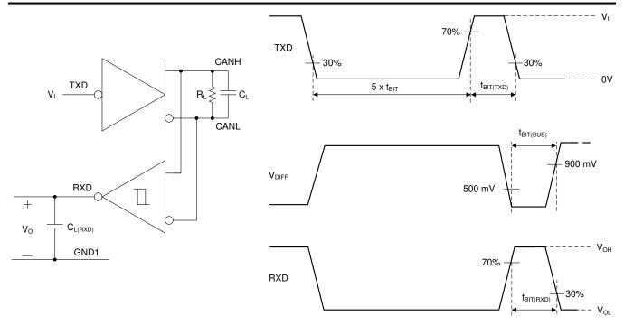
Figure 7-7. CAN FD Timing Parameter Measurement
