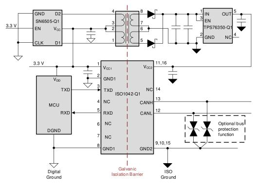
Figure 9-1. Application Circuit With ISO1042-Q1 in 16-SOIC Package
