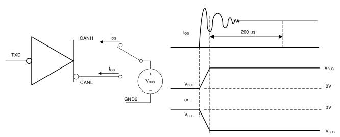
Figure 7-9. Driver Short-Circuit Current Test Circuit and Waveforms
