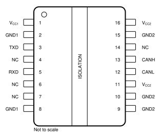
Figure 5-1. DW Package 16-Pin SOIC Top View
