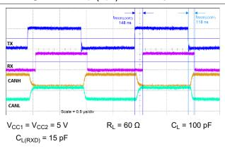
Figure 6-12. Typical TXD, RXD, CANH and CANL Waveforms at 1 Mbps
