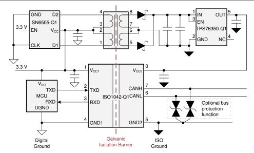
Figure 9-2. Application Circuit With ISO1042-Q1 in 8-SOIC Package
