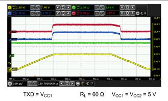
Figure 6-14. Glitch Free Power Up on V<sub>CC2</sub> – CAN Bus Remains Recessive
