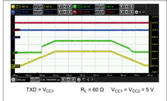
Figure 6-13. Glitch Free Power Up on V<sub>CC1</sub> – CAN Bus Remains Recessive
