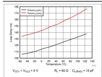
Figure 6-9. Loop Delay vs Ambient Temperature
