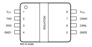
Figure 5-2. DWV Package 8-Pin SOIC Top View
