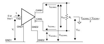
Figure 7-1. Driver Voltage, Current and Test Definitions
