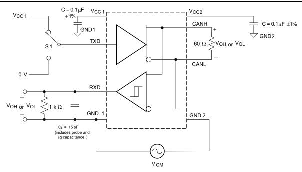
Figure 7-10. Common-Mode Transient Immunity Test Circuit
