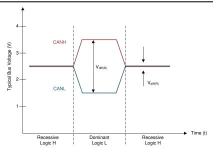
Figure 8-1. Bus States (Physical Bit Representation)
